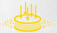
Pushing (or pulling) some times the lateral flap and closing the suction intake at the same time, it is possible to get an immediate filter cleaning, thanks to the differential pressure generated. This simple operation guarantees the maximum filtration capacity and best vacuum cleaner performance.
